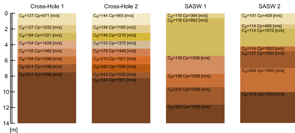
Figure 1 - Comparison of soil mechanical properties obtained through Cross-hole and SASW tests carried out on site.[5].
