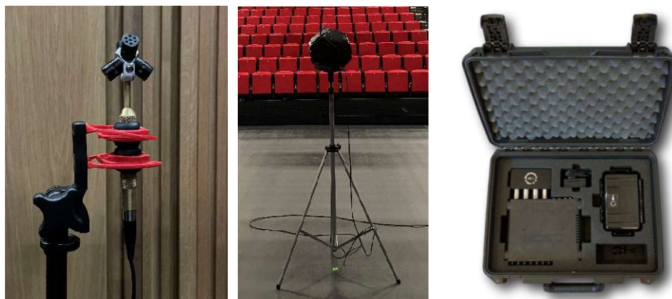
Figure 6 – Measurement equipment: TetraMic (left), dodecahedron loudspeaker (middle), IRIS kit (right)
