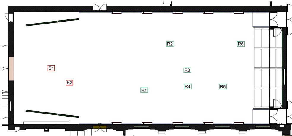
Figure 7 – Receiver (green) and source (red) positions
