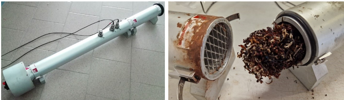
Figure 5 – Apparatus for measuring the sound absorption coefficient at normal incidence and sample mounting method
